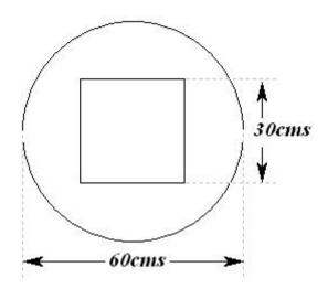
The sketch above shows a component which is stamped out of sheet steel. The square in the center is discarded. These components are stamped out of a continuous steel coil with a width of 70 cms. The stamping process requires a gap of 25mm between each component. The steel coil is supplied in lengths of 25 meters costing \$200.
